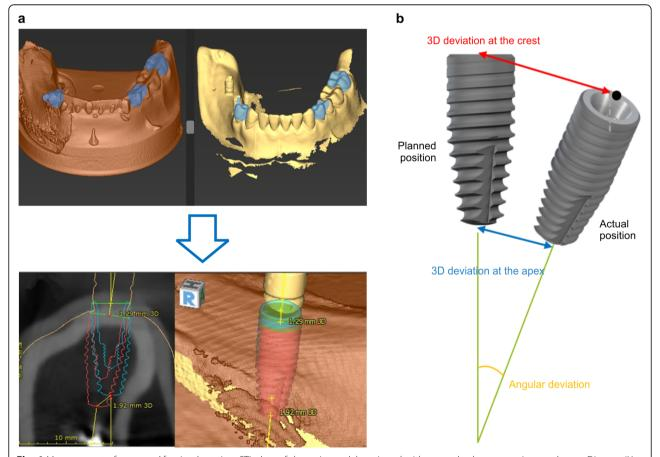
**Fig. 4** Measurement of errors. **a** After implantation, STL data of the resin model equipped with a scan body are superimposed on coDiagnostiX simulation data. Accuracy was measured using the treatment evaluation tool. Blue: implantation position set using simulation. Red: implanted position. **b** Evaluation of deviation measurements
