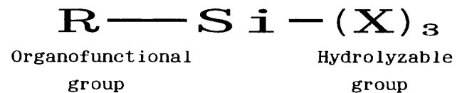
Fig 1 Structure of Silane Coupling Agent
